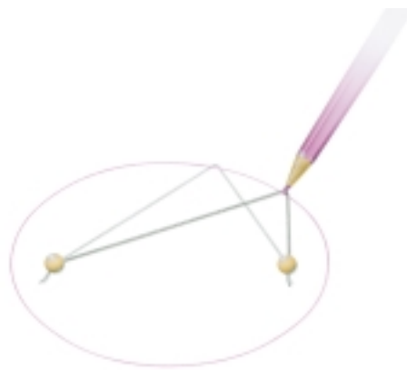
Figure 1 An ellipse can be drawn using two pins and a string.
